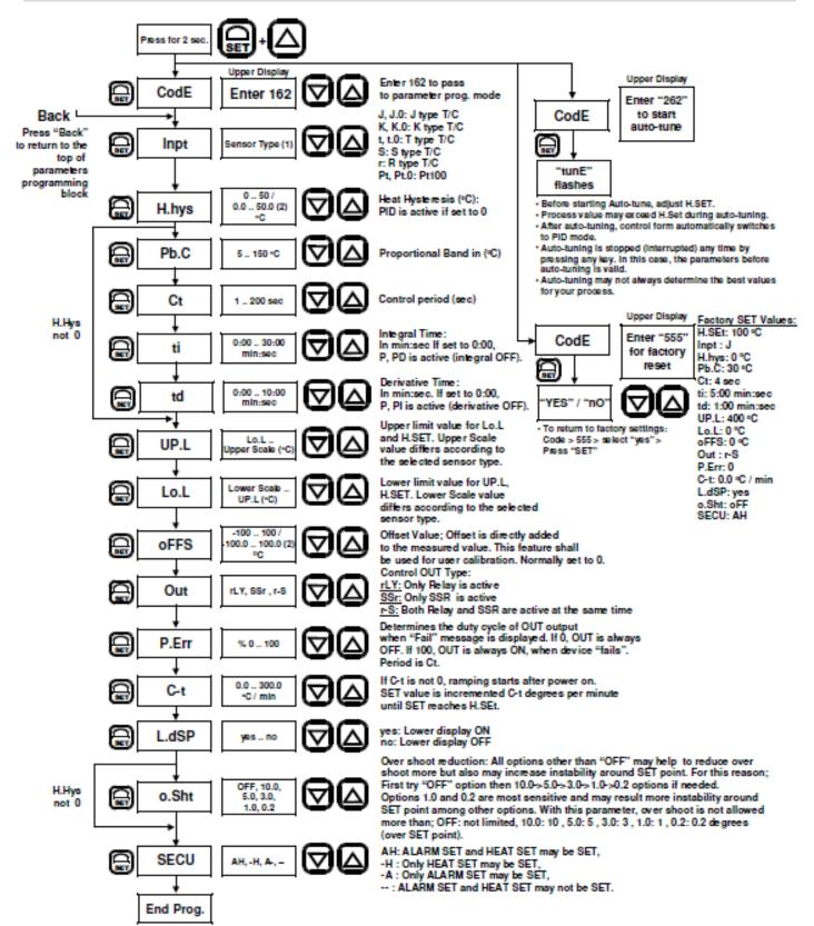
(1)When sensor type is changed, Up.L, Lo.L, H.Set, H.hys, oFFs may be set to a new value automatically, according to the selected sensor. (2) If sensor type is selected as Pt.0, J.0, K.0 or t.0.
