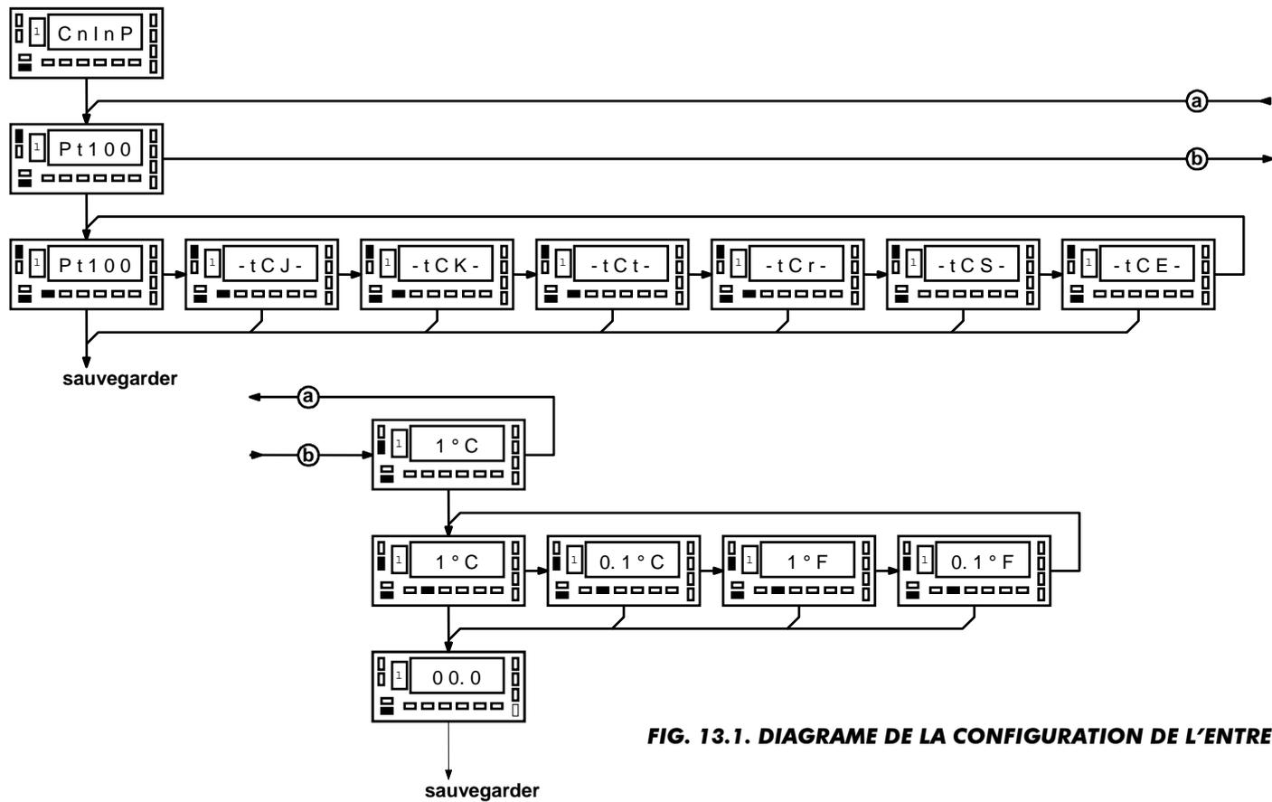
**FIG. 13.1. DIAGRAMME DE LA CONFIGURATION DE L'ENTREE**
